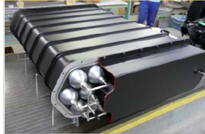
2nd-generation High-pressure Hydrogen absorbing Alloy Tank.
